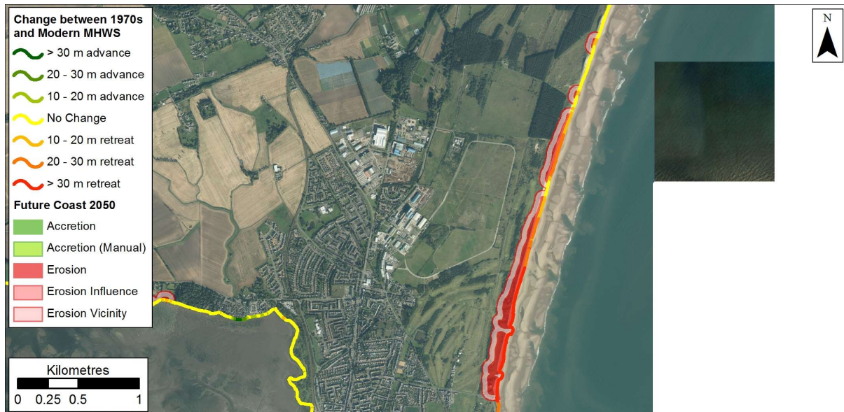
Figure 2.20: Possible future coastline position in 2050 based on rates between 1970 and Modern MHWS data at Montrose. Getmapping are our current providers of Scotland-wide digital aerial imagery © Getmapping plc.
