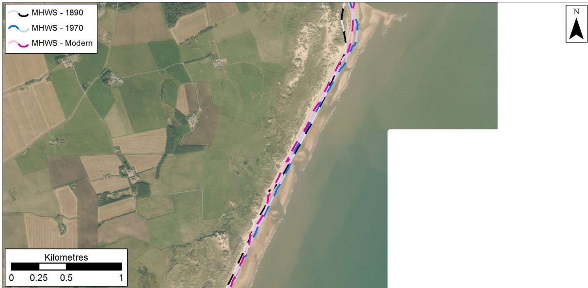
Figure 2.26: MHWs position in 1890, 1970s, and Modern datasets south of the River Ythan mouth. Getmapping are our current providers of Scotland-wide digital aerial imagery© Getmapping plc.
